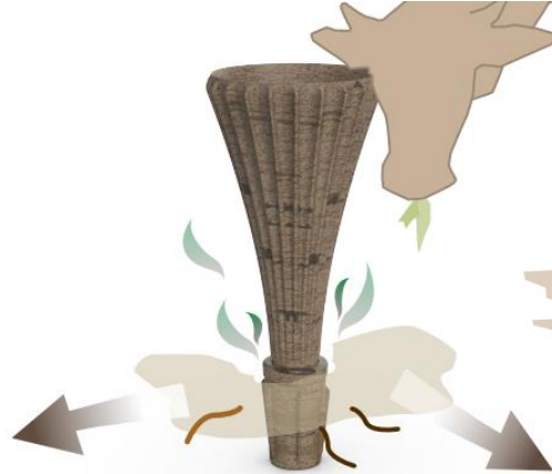
11. The height of the outer layer is designed to prevent livestock from biting it, and the application of bitter oil serves to prevent insect infestations.
